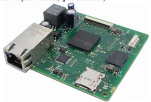
The MP1 is already well supported by the Barebox bootloader and the mainline kernel, and, as it has the same Vivante 3D GPU family as many i.MX processors, it also runs the open source 3D graphics driver suite provided by Etnaviv.
